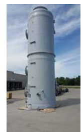
Right Photo: Perry 15,000 cfm chemical scrubber. Perry supplied; controls, pumps, fans, packing and chemical feed pumps.
